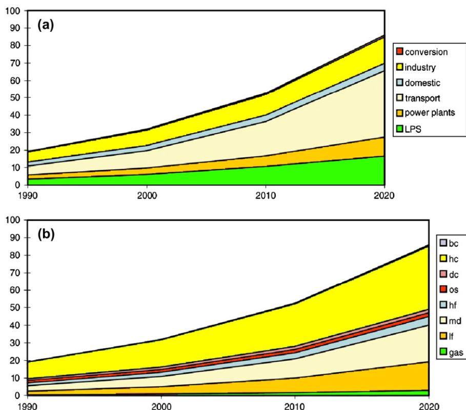
Fig. 3.  $\text{NO}_x$  emissions by economic and fuel type in the period 1990–2020 ( $\text{NO}_2 \text{ yr}^{-1}$ ) (Van Aardenne et al., 1999).
