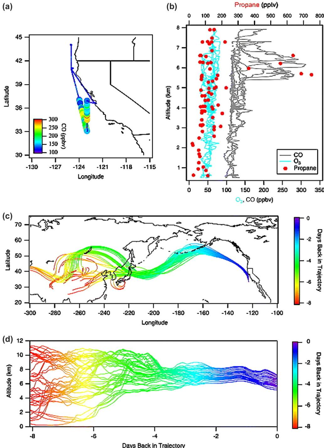
Fig. 4. (a) The 5 May flight track colored by the CO observations with the large markers, indicating the intersection of the transport plume. (b) Altitude (km) versus O<sub>3</sub> (teal) and CO (gray) on the bottom axis and propane (red circles) on the top axis above 0.5 km for the whole flight. (c) The 8-day back trajectories associated with the intersected plume colored by the number of days back along the trajectory. (d) Altitude of the back trajectories (Nowak et al., 2004).
