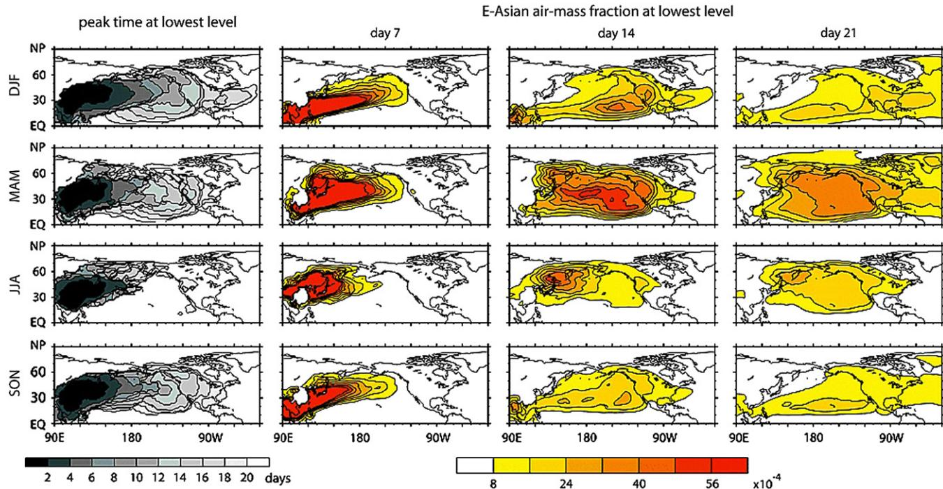
Fig. 7. Leftmost panels: The peak time of the climatological E-Asian air-mass fraction at the surface (lowest model level) for all four seasons, as indicated. Colored panels: The climatological air-mass fraction at the surface that had its last contact with the E-Asian source region during the 24-h periods 7, 14 and 21 days ago, as indicated for each season (Holzer et al., 2005).
