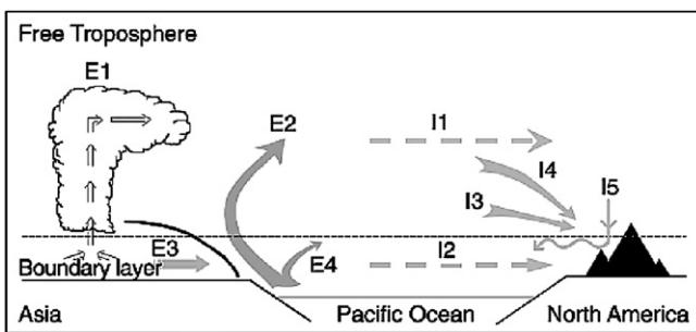
Fig. 5. Schematic of export mechanisms over east Asia and import mechanisms over the NE Pacific for long-range transport of Asian pollutants (Liang et al., 2004).
